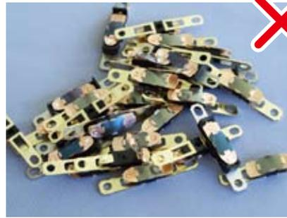
If you put thermostats on workbench randomly, contacts and terminals might get stuck each other. Such conditions may decrease contact pressure or keep contacts open always. If contacts keep open, it will result in non-energizing final application.
