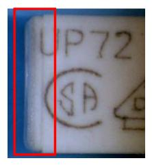
Different Press Joint Shape of Resin Molding
